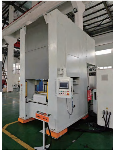
STSZG1 TYPE HIGH RIGID SERVO STRAIGHT SIDE SINGLE POINT HIGH PRECISION COINING PRESS
